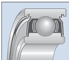
Flexeals are recommended in applications where contamination is generated around the bearing or in equipment which must operate in a contaminated environment.
