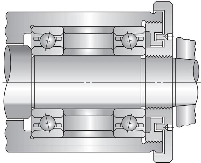
Fig. 7: Duplex bearing pairs with equal width spacers.
