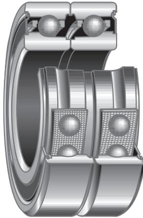
Preload increase at the higher speeds is always a problem with high speed spindles due to the heat generation when solid preloading is used. Therefore, another major advantage of the 25° contact angle is a much lower preload increase at high speeds when compared to the 15° bearing, due to the favorable internal geometry.
