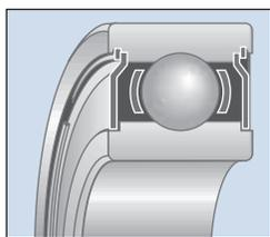
contoured configuration to provide strength and rigidity, resistance to vibration, and positive radial and axial positioning against the shield shoulder in the outer ring.
