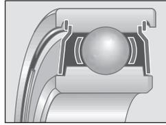
Detail close-up showing how Flexeal Seals provide sealing action. If it is necessary to use a single Flexeal, indicate by using a single suffix "F" in the bearing number.
