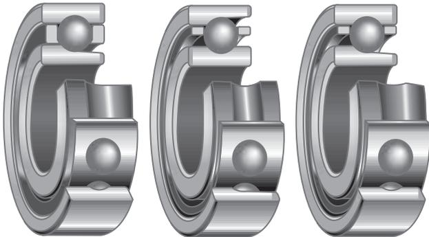
**Separable Type B:** Outer ring has full shoulders, inner ring has one shoulder cut away. Inner ring is removable for mounting on the shaft separately from the outer ring assembly.
