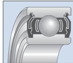
The barseal is a molded rubber seal which incorporates a metal stiffening insert. This design provides maximum volume within the bearing for lubrication. Speed considerations limit their use to
