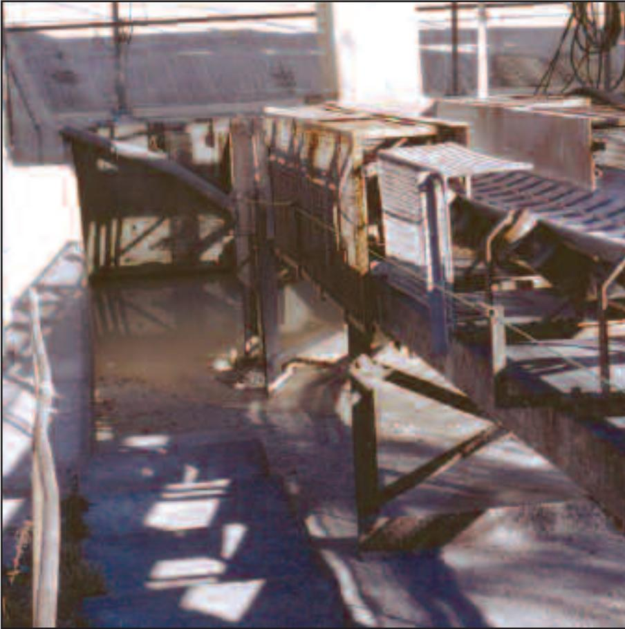
Water collected in the tail drum pit and entered the tail drum bearings. As a result, the SNL 515 - 612 bearing fitted to the 100mm shaft failed every 2 to 3 months.
